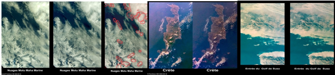
Figure 2: Left: clouds over the Motu Maha Marine, of the south of New Zealand. Without stereoscopic pictures, it is difficult or impossible to distinct clouds and their altitude. Thanks to 3d, (third picture) we can spot in red the clouds that are a layer above the others.
